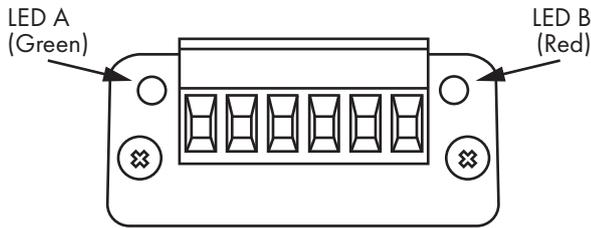
If either LED is not illuminated, the corresponding sensor is not connected correctly or damaged. Check that the connections are made correctly as shown above or replace the sensor.
