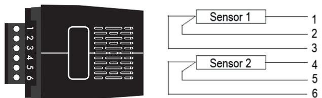
**NOTE** To minimise on any noise injection into the drive control circuit, ensure that the PT100/PT1000 sensors connected are isolated from power earth (ground).
